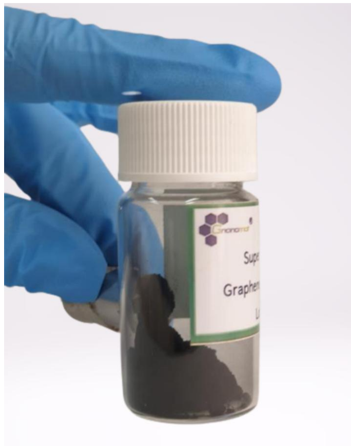
Fig. 14 Gnanomat's Superparamagnetic Graphene hybrid powder reacting to a magnetic field.
