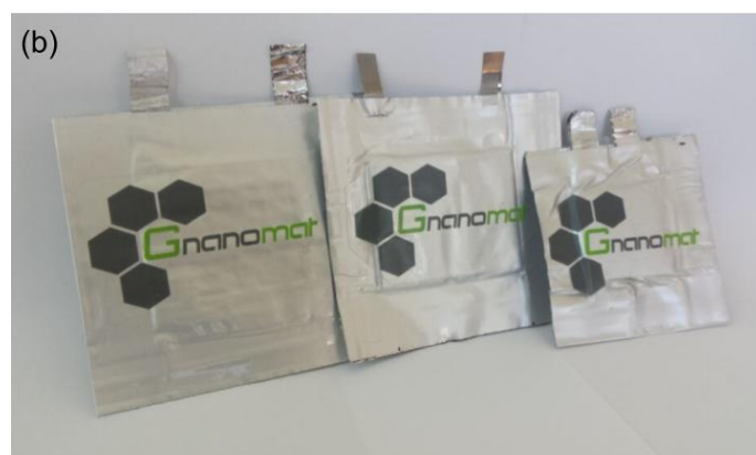
Fig. 9 (a) Improvement of Gnanomat asymmetric pseudocapacitor (PSEU-GNM) cells compared to a standard EDLC cell. (b) Photograph of manufactured pouch cells.
