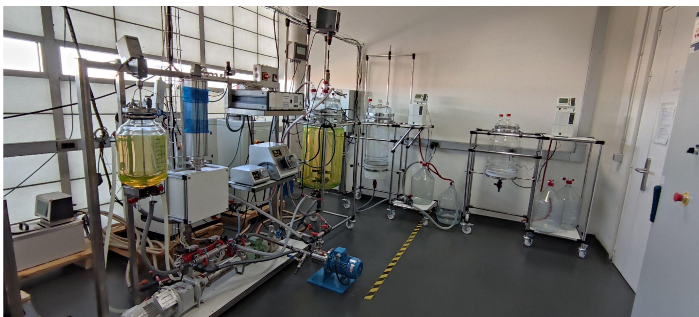
Fig. 4 Gnanomat's pilot plant for hybrid nanomaterial production.
