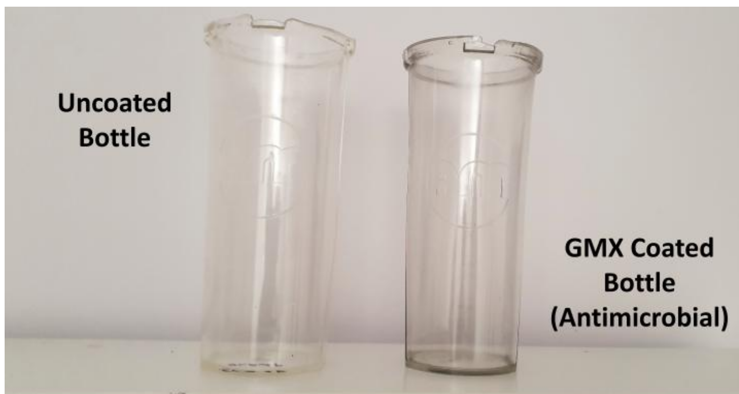
Fig. 11 Optically transparent antimicrobial coatings developed using Gnanomat's hybrid nanomaterials.
